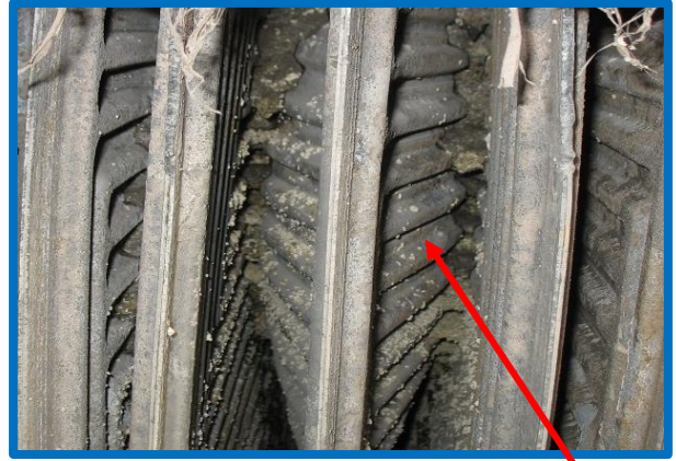
Example of actual "zippered" failure
